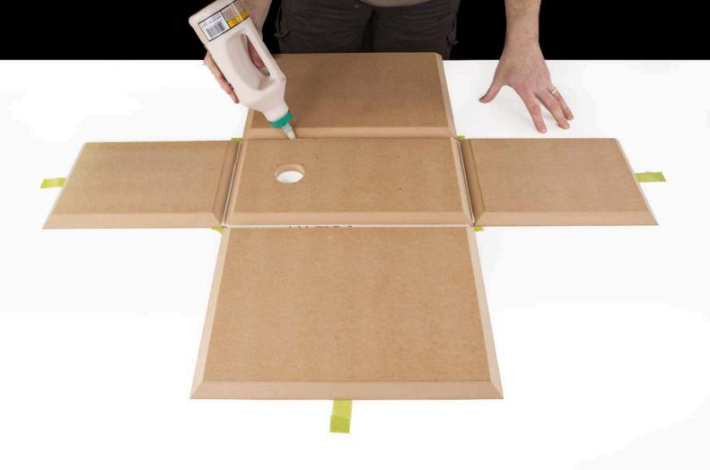
Apply a glue bead to all four joins between the rear and adjacent panels. This first bead of glue should be applied to the bottom of the mitre. Then apply a second bead in the middle of the mitre. This bead should be thicker than the first, as you can see below.
