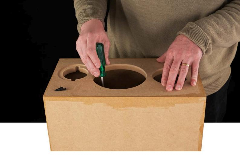
As shown above, driver cutouts provide access to fix the passive crossover board in place. Using the shorter screws, fix the board in place with a Phillips head screwdriver. Avoid over tightening. Ensure the board is oriented so the inputs with the shortest cable pair are near the terminal cut out.
