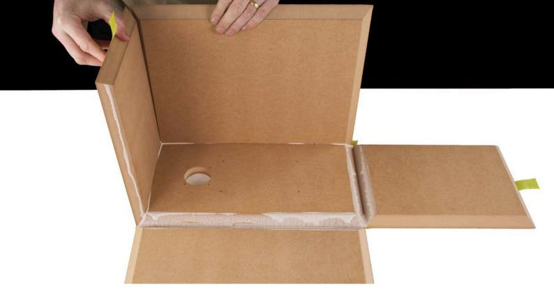
Confirm that the glue adequately covers the entire surface of the joins by folding up each pair of panels. Check the glue covers the entire surface and add more glue where necessary. Now apply glue to the joins between top, bottom and side panels.
