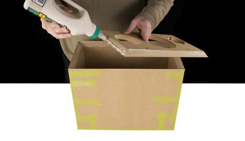
Apply one thick glue bead to the mitres on the front baffle. Confirm the amount of glue by pressing into position. The entire join should be covered in glue – apply more glue where necessary. The photo above shows a second bead being applied after checking the glue cover.
