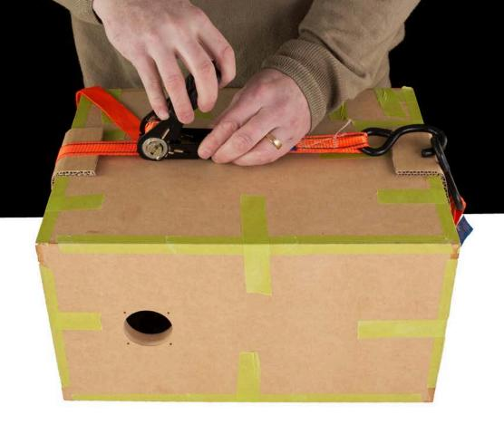
An optional step for improved clamping pressure is to secure top, bottom and side panels with a tie down ratchet strap. Avoid damage to the surface of the MDF by placing cardboard strips under the straps at all four corners. Be careful to avoid applying excessive force, which can damage the corners of the MDF or even collapse the cabinet.
